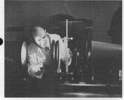
STRESS LINES IN PLASTIC are revealed by the polaroscope which throws a technicolor picture on a screen. Shown here adjusting the scope is Les Neeves, 1514-3. Light passing through a thick sheet of plastic set between a series of lenses projects a view of the plastic's internal flaws.
